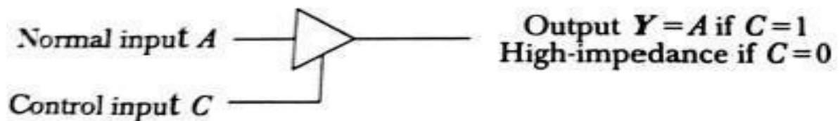
Figure 4-4 Graphic symbols for three-state buffer.
