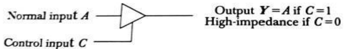
Figure 4-4 Graphic symbols for three-state buffer.
